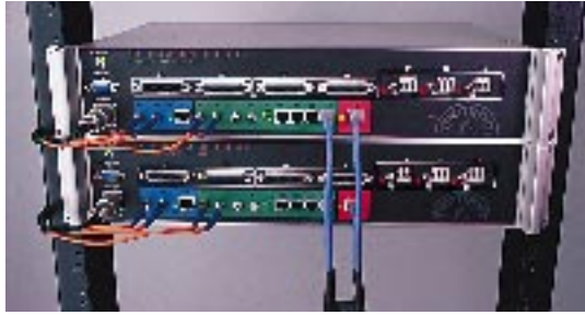
Network interface units, either wayside or carborne, translate the train control messages between native and IP format.
